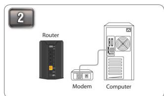
Turn off and unplug your cable or DSL Position your router close to your modem and a computer. Place the router in an open area of your intended work area for better wireless coverage.
